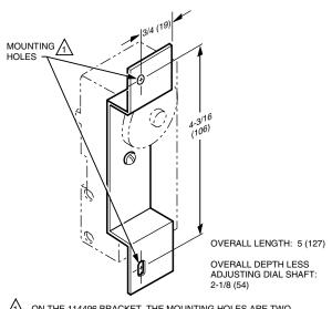
ON THE 114496 BRACKET, THE MOUNTING HOLES ARE TWO NO. 8-32 TAPPED HOLES. THE 107940 BRACKET IS MOUNTED WITH A 5/32 (4) DIAMETER HOLE AT THE TOP AND A VERTICAL 5/32 X 5/16 (4 X 8) SLOT AT THE BOTTOM.
