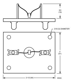
Fig. 2. Approximate dimensions of C7150B Mixed/ Discharge Air Sensor in in. (mm).
