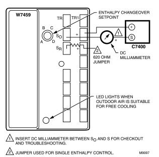
Fig. 20. Location of enthalpy setpoint potentiometer, minimum position potentiometer and LED.
