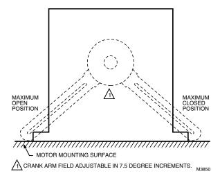
Fig. 9. Limits of crank arm rotation.
