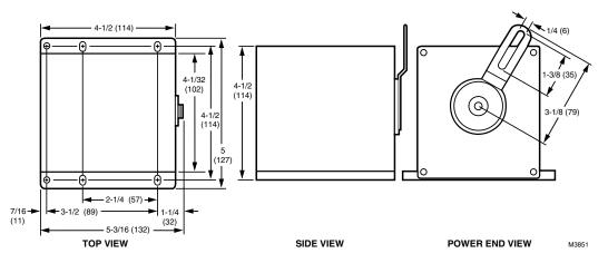
Fig. 4. Approximate dimensions of M7415A and M8405A in in. (mm).
