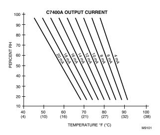
Fig. 16. C7400A Sensor output current vs. relative humidity.
