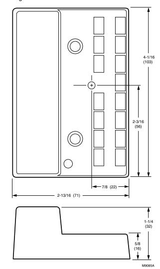
Fig. 6. Approximate dimensions of W7459 Solid State Economizer Logic Module in in. (mm).
