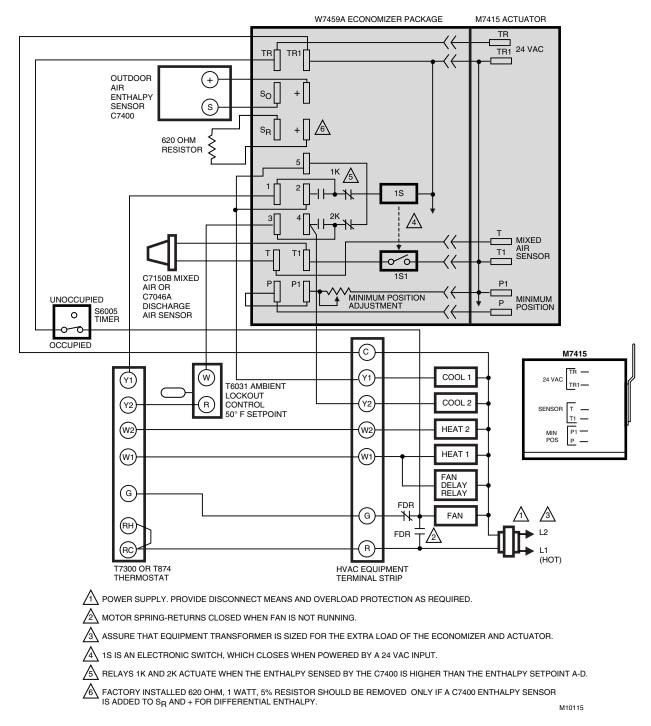
Fig. 13. W7459A, D/C7400 used in two-stage cooling system with single enthalpy changeover and with M7415 Actuator.
