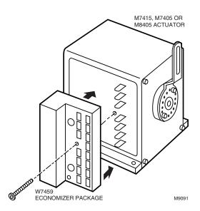
Fig. 12. Mounting W7459 on M7415 or M8405 Damper Actuator.
