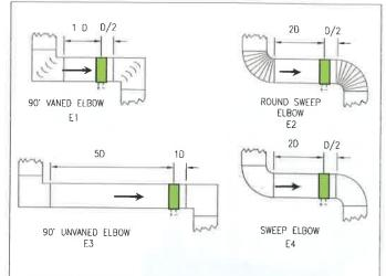
Air measurement can be more accurate and less problematic when air measurement considerations are accounted for in the mechanical specification and building design. The acceptable placement of an air measurement device is shown in green.
