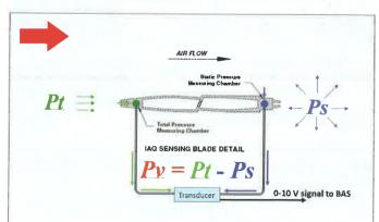
∼ Velocity pressure explained through a cross-section
