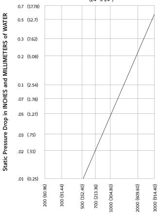
Air Velocity in FEET and METERS per minute through FACE AREA. Tested per AMCA Std. 500, Fig. 5.3, ductwork upstream and downstream.
