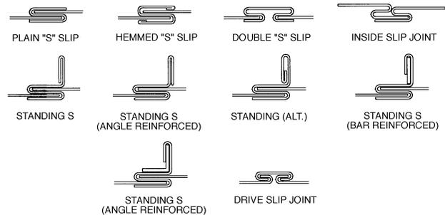
A maximum of two #10 (M5) sheet metal screws on each side and the bottom, located in the center of the slip pocket and penetrating both sides of the slip pocket may be used. Connections using these slip joints on the top and bottom with flat drive slips up to 20" (508) long on the sides may also be used.
