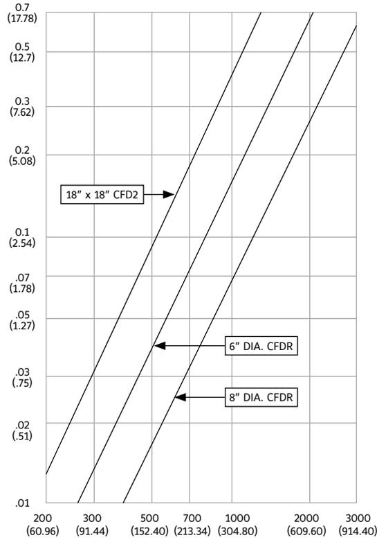
Air Velocity in FEET and METERS per minute through FACE AREA.
