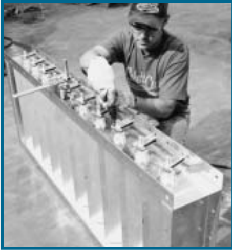
Operating linkages can be located in-airstream or mounted as side linkage for routine maintenance and inspection.
