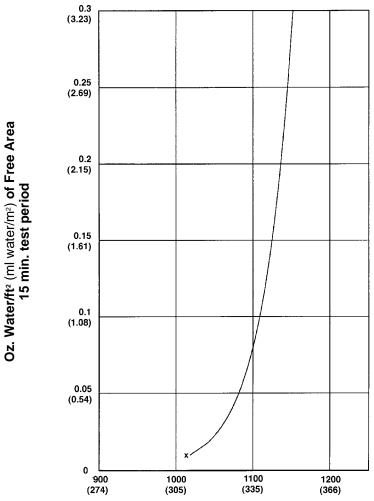
Free Area Velocity in feet (meters) per minute Standard air .075 lb/ft³
