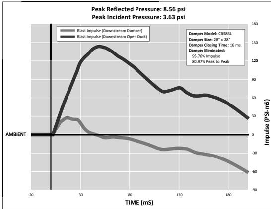
Ruskin blast damper charts below highlight results of independent third party lab testing of model CBS8BL to peak reflected pressures of 8.56 psi and 38.4 psi, respectively. The results show that Ruskin's CBS8BL dramatically reduces the blast impulse, thus protecting downstream equipment and components.
