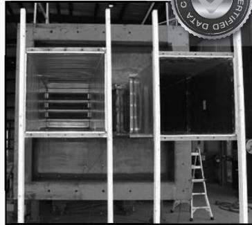
The Ruskin model CBS8BL blast damper performance has been evaluated by an independent firm via blast testing in shock tubes using several test configurations. The data shown above is representative of the results of the testing. The testing included simultaneously applying blast load to two duct openings, with one duct protected by a damper and the other unprotected.
