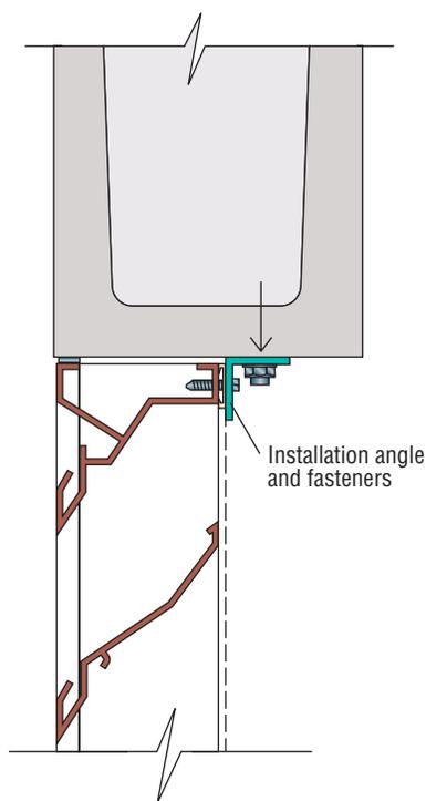
**FIGURE 2. Installation-angle attachment.**
