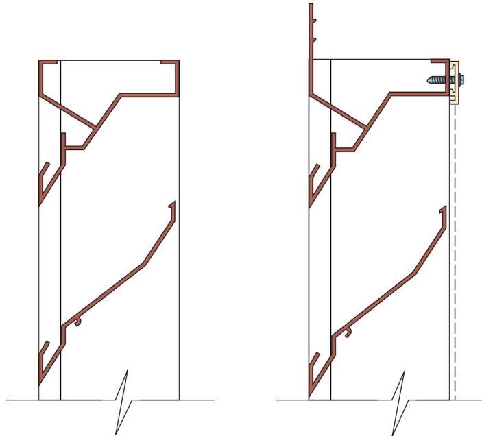
**FIGURE 1. Channel frame (left) and front-flange frame (right).**
