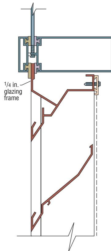
**FIGURE 3. Louver installation with a  $\frac{1}{4}$ -in. glazing frame.**
