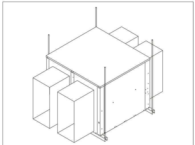
5. When hanging from the structure (usual installation) proper rigging should be used, Unistrut or angle iron is suitable along with (minimum) 3/8ths all-thread. Prepare rigging before lifting unit making sure that ERV will be supported at the 4 corners and that access panels will not be blocked.
