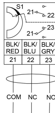
Auxiliary Switch Wiring Diagram
