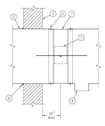
SD34, SD35, SD36, SD37, SD50, OR SD60 MULTIPLE BLADE LEAKAGE RATED DAMPER INSTALLED WITHIN A DUCT OR SLEEVE (SD50/SD60 SHOWN)
