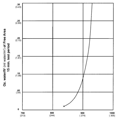
Free Area Velocity in feet (meters) per minute Standard air .075 lb/ft³ (1.2 kg/m³)
