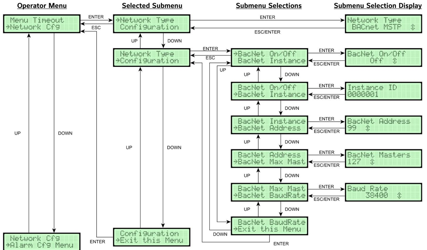
**Firmware Note:** Only **ONE** Network output configuration can be active at a time.
