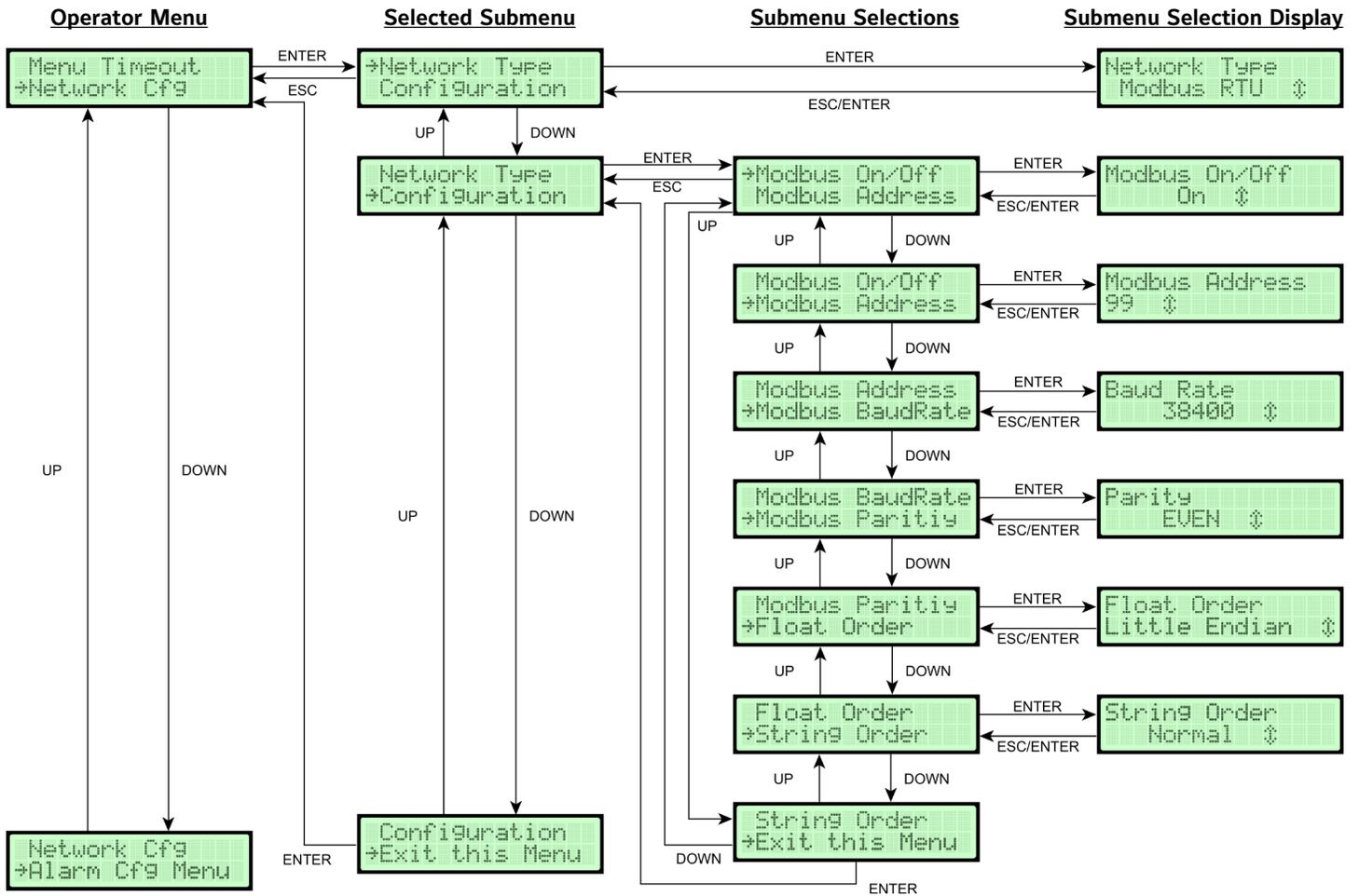
**Firmware Note:** Only **ONE** Network output configuration can be active at a time.
