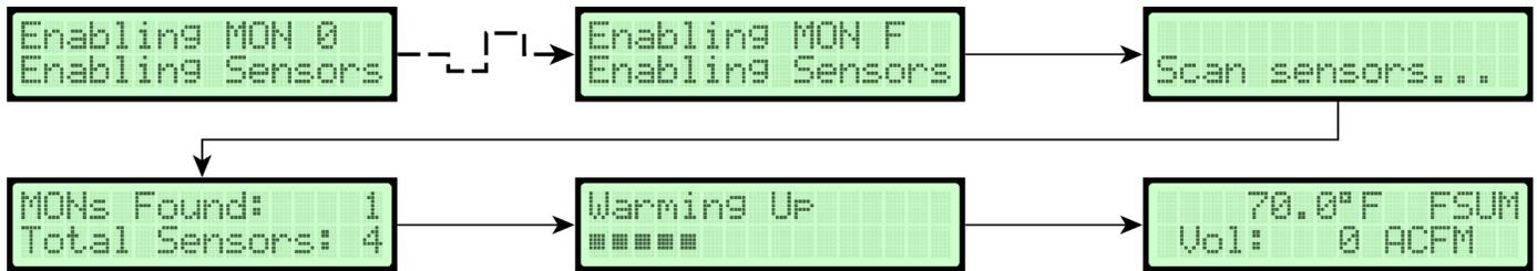
4. The TDFi-FA system will automatically reset all settings to default, all sensors, and devices, then restart and warm-up. Then returns to the Normal Operational Mode. All settings will be returned to a default state from the factory.
