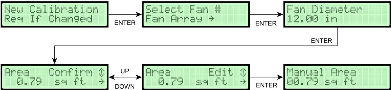
4. Use UP or DOWN to change setting. Once desired setting is displayed, press ENTER. New setting will be stored in memory and display will progress through the required values for the shape selected and save each value as they are confirmed. With all required values entered the display will return to the Flow Configuration Menu shown in Step #2.
