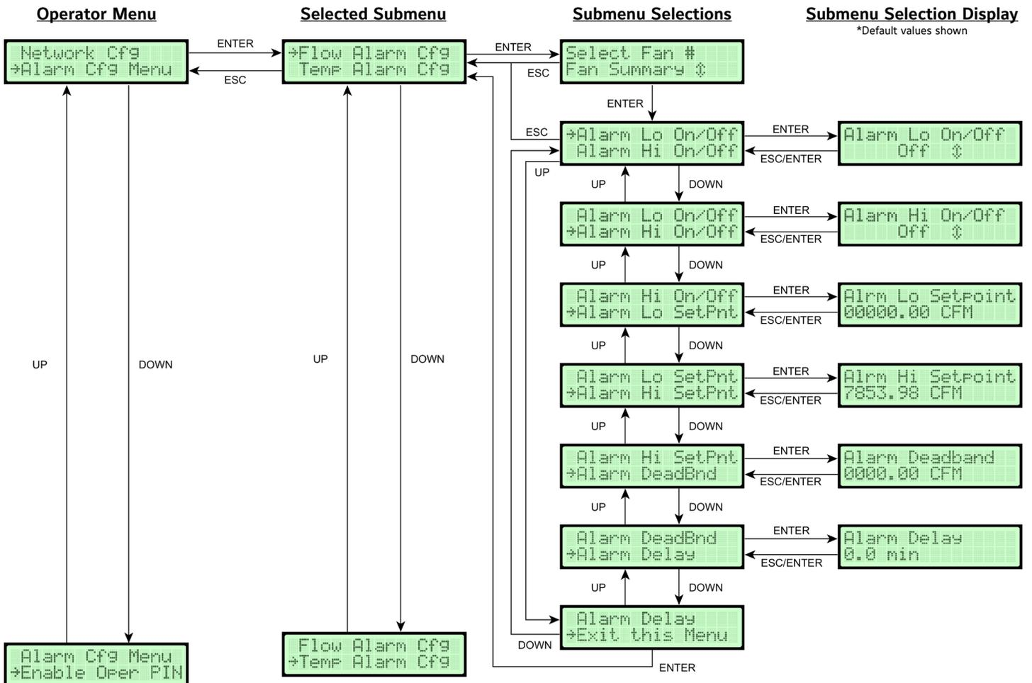
1. In the Operator Menu, press UP or DOWN to scroll to the RS-485 interface Flow Alarm Configuration submenu.
