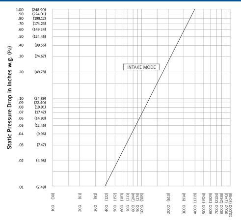
Air Velocity in feet (meters) per minute through Free Area NOTE: Ratings are based on AMCA Standard 610 Test Setup Figures 1 & 2. Ratings do not include the effect of a bird screen.
