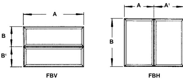
Dampers larger than maximum single section are an assembly of equal size single section dampers (maximum section size 48"w x 72"h [1219 x 1829]) and may be coupled for operation in a variety of ways. A 1" (25) diameter jackshaft is normally used for multiple section coupling as illustrated above.
