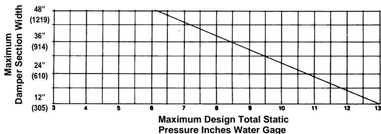
The CD403 dampers may be used in systems with total pressures exceeding 6" w.g. by reducing damper section width as indicated. Example: Maximum design total pressure of 8.5" w.g. would require the CD403 damper with Maximum Section Width of 36" (914).
