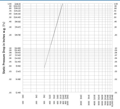
Air Velocity in feet (meters) per minute through Free Area Maximum recommended free area intake velocity through louver: 550 fpm (168 m/min).
