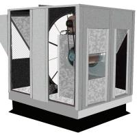
"S" Series energy recovery ventilators are designed for outside use in rooftop or "pad" installations where the application requires a "side-byside" duct system. One of the benefits of this design is the ability to easily be connected to the horizontal ductwork of an air conditioning system. Balancing dampers should be utilized to help control the air volumes.
