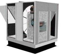
"0" Series energy recovery ventilators are designed for outside use in rooftop or "pad" installations where the application requires an "over and under" duct system. One of the benefits of this design is the ability to be ducted directly to the back of a rooftop air conditioning unit. Another use is for "through the wall" applications. The horizontal return duct connection can be converted to bottom return in the field. Balancing dampers should be utilized to help control the air volumes.
