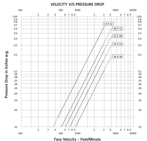
CD450V sizes 12 x 12, 24 x 24, 48 x 12, 12 x 48, 36 x 36 (305 x 305, 610 x 610, 1219 x 305, 305 x 1219, 914 x 914) All data corrected to represent standard air at a density of  $0.075 \text{ lbs/ft}^3$ .
