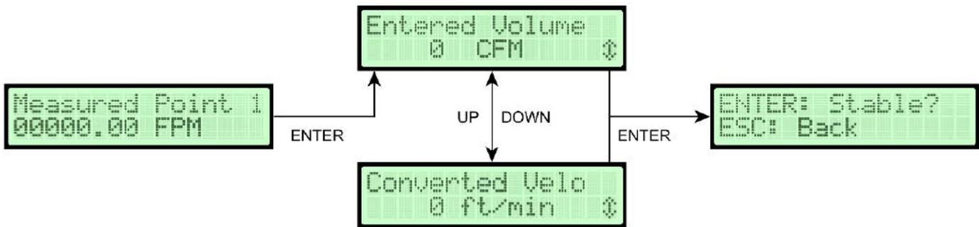
6. The device will compare the entered value to the sensor readings for each sensor and display the values. When Sensors per Fan is set to 1, only one comparison will be displayed.
