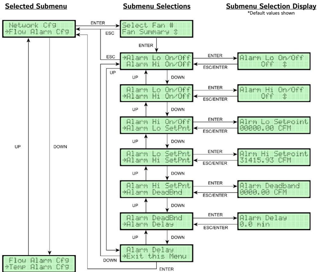
1. In the Operator Menu, press UP or DOWN to scroll to the RS-485 interface Flow Alarm Configuration submenu.
