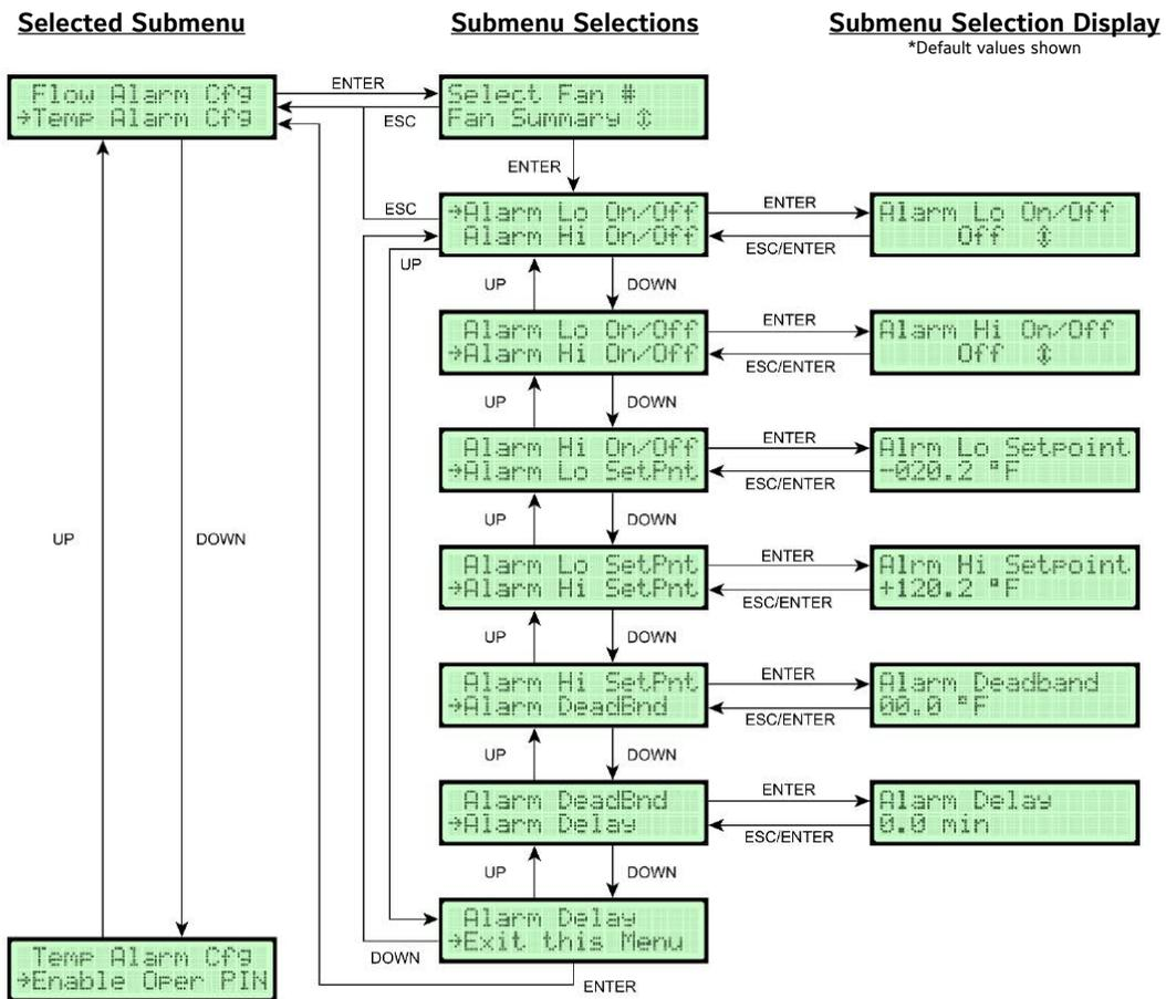
1. In the Operator Menu, press UP or DOWN to scroll to the RS-485 Interface Temperature Alarm Configuration sub-menu.
