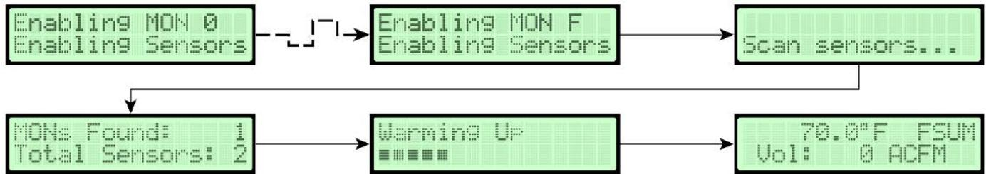
4. The TDFi-Rt system will automatically reset all settings to default, all sensors, and devices, then restart and warm-up. Then returns to the Normal Operational Mode. All settings will be returned to a default state from the factory.
