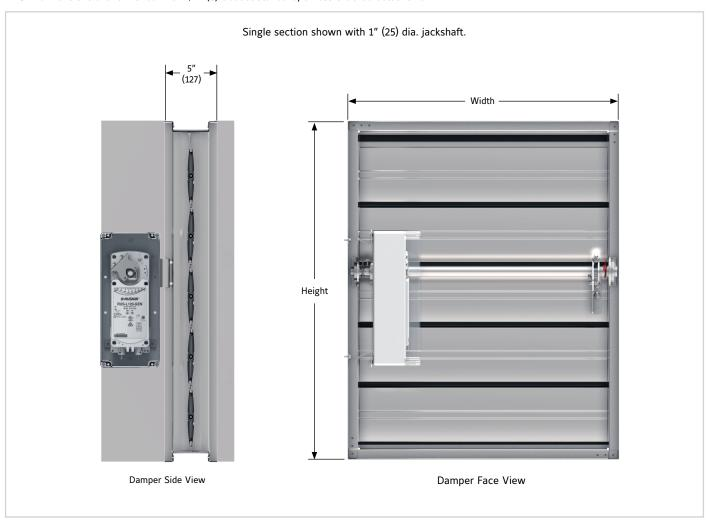
Note: Minimum damper size for internal actuator & weather enclosure is 18" X 30" (457 X 762)
