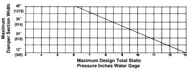
The CD403 dampers may be used in systems with total pressures exceeding 6" w.g. by reducing damper section width as indicated. Example: Maximum design total pressure of 8.5" w.g. would require the CD403 damper with Maximum Section Width of 36" (914).
