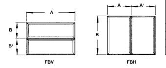
Dampers larger than maximum single section are an assembly of equal size single section dampers (maximum section size 48"w x 72"h [1219 x 1829]) and may be coupled for operation in a variety of ways. A 1" (25) diameter jackshaft is normally used for multiple section coupling as illustrated above.
