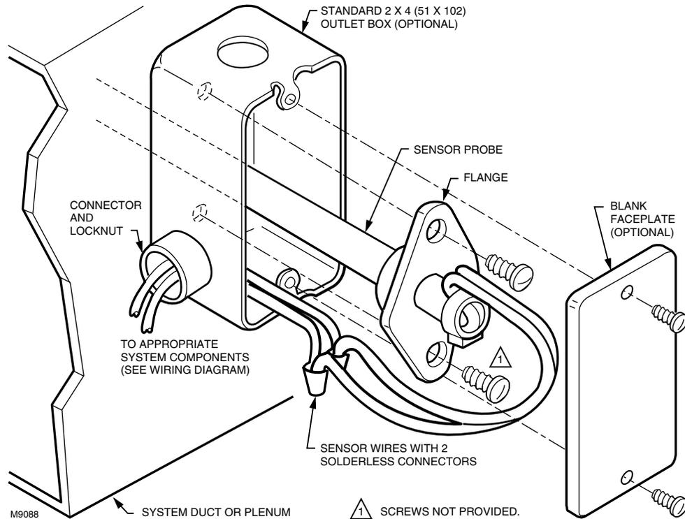
Fig. 8. Mounting C7046C Discharge Air Temperature Sensor in junction box.
