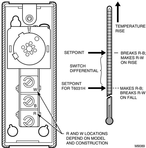
Fig. 11. T6031H switch terminal arrangement and switching.
