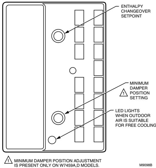
Fig. 20. Location of enthalpy setpoint potentiometer, minimum position potentiometer and LED.
