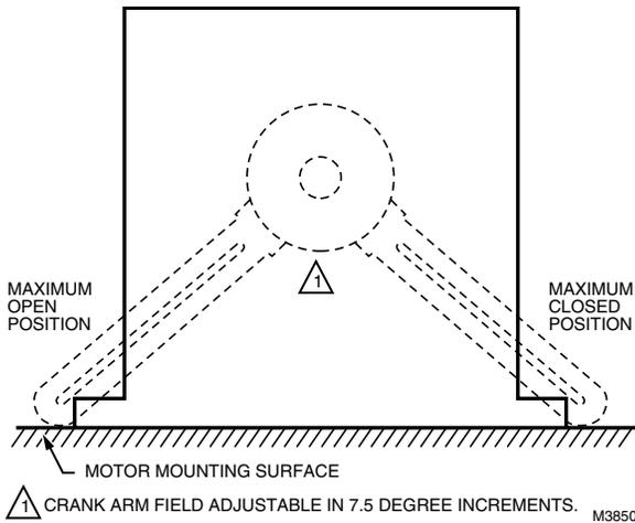
Fig. 9. Limits of crank arm rotation.
