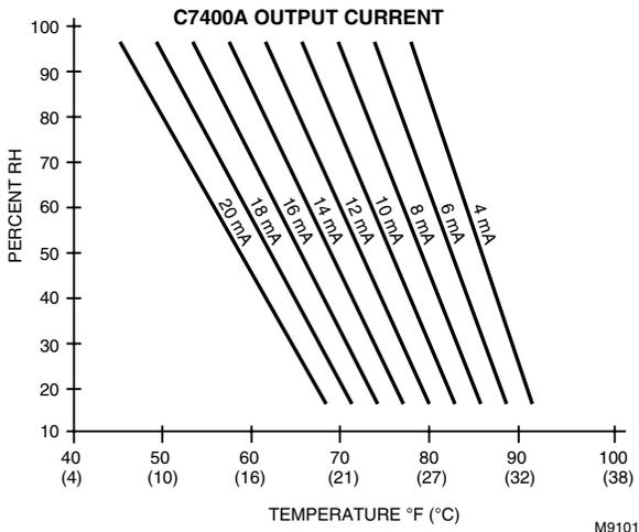
Fig. 16. C7400A Sensor output current vs. relative humidity.
