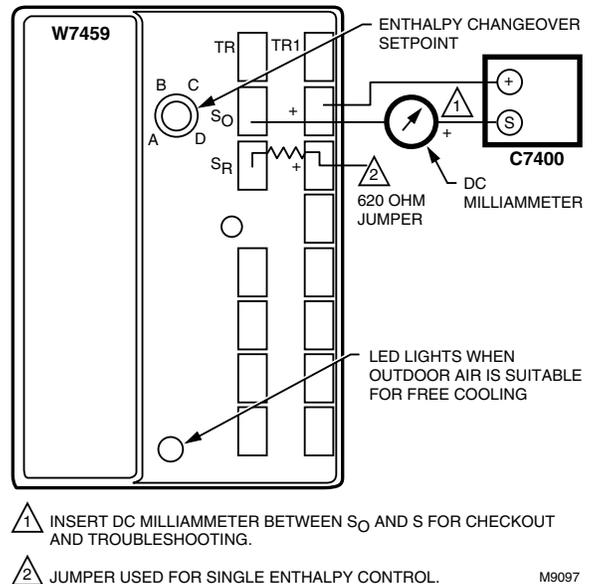
Fig. 21. Meter location for checkout and troubleshooting.
