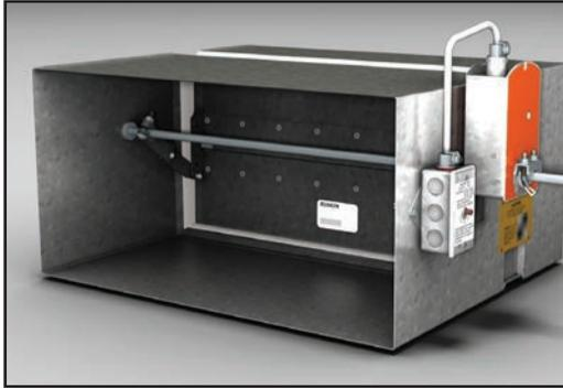
Ruskin FSD60LP, FSD60LP-2, FSD37LP and FSD36LP ultra low leakage, low profile and low pressure drop combination fire and smoke dampers provide point-of-origin fire and smoke containment. The FSDLP series is provided with an integral sleeve/frame design to obtain the pressure drop of less than .03 at 1000 FPM (5.1 m/s). All FSD60 series dampers may be installed vertically in walls, or horizontally in masonry floors, and are rated for airflow and leakage in either direction.
