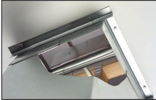
Ductwork may be connected directly to the bottom side of the CFD7(T) from the AHU below. Retaining angles are utilized in lieu of steel grille flange that cover the gap in between the gypsum and the CFD7(T).
