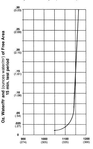
Free Area Velocity in feet and (meters) per minute Standard air .075 lb/ft<sup>3</sup>
