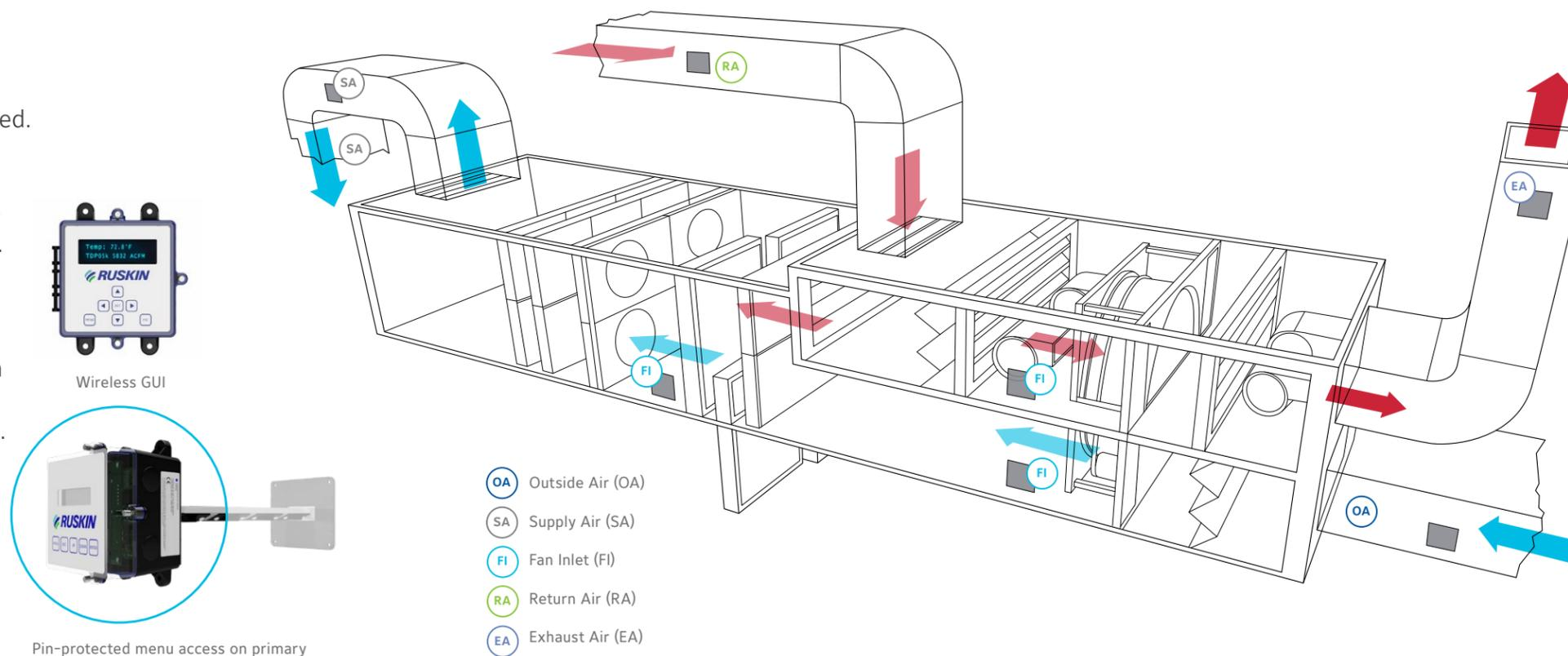
**Every air measurement station** has a primary. It can be located on the end of the probe, as shown above or as a separate box remotely located up to 500 feet away from the air measurement station. The primary displays airflow and temperature during normal operation and allows easy menu access without removing covers or screws. The Remote Graphic User Interface (GUI) provides the same display and menus, wired or wirelessly.
