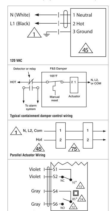
Auxiliary Switch Wiring
